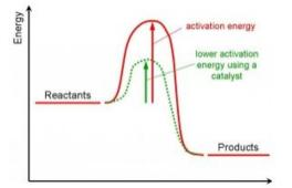
Catalysts provide a different pathway for a chemical reaction that has a lower activation energy.
